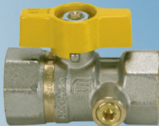
Art 4094 F/F NPT with sealed side tap. Available range from 3/8" to 3/4"
